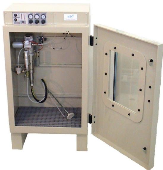
***Automatic electrostatic system for water based paints, with insulation and medium pressure feeding. Can be used with high viscosity fluids, with stainless steel tank (optional). Stainless Steel Pump lower and fluid passages suitable for water base paints. Innovative electrostatic system with product, air, and voltage adjustments outside the cabinet. Automatic cleaning system, (optional).***
